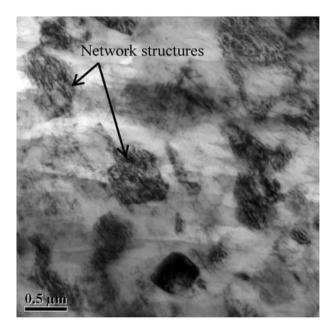
Fig. 4 TEM micrograph of the AZ31 Mg alloy processed by the CEC method after 6 passes showing the network structures
